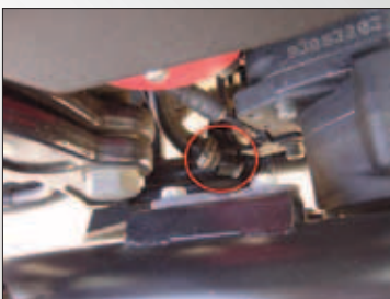
Touring models, don't remove the wrong plug! Oil is the one facing forward NOT down.
