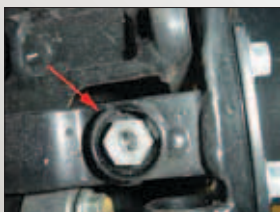
Older Softail on the right side, remove plug from oil line.
