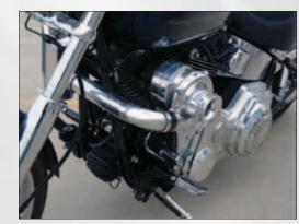
Fig 3 Procharger centrifugal supercharger setup
