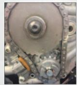
Fig 6 The NEW bottom gear that drives the Blower unit... simple and reliable with lots of tolerance for the Harley Twin Cam crank run out problems!
