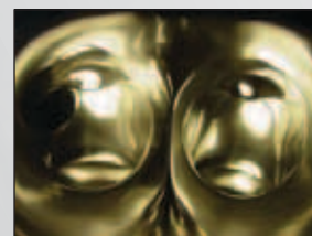
Fig 3. Way to polished for an intake port, you must have turbulence too!
