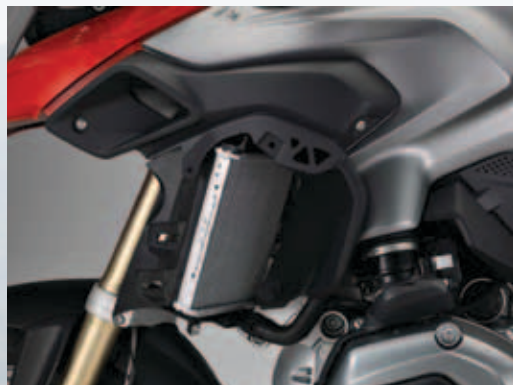
A subtle radiator cools a glycol-water blend that is then circulated through key, high temperature parts of the engine
