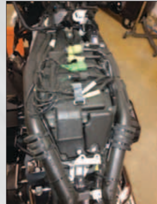
Fig 2 Fuel tank off ready for disassembly
