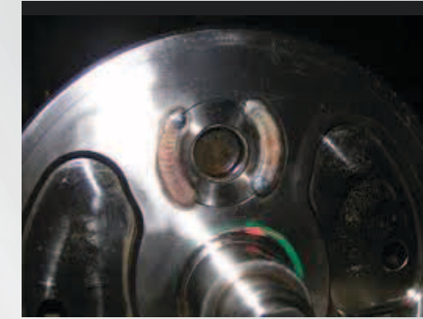
Fig 7 Welded crank pin, no more movement!
