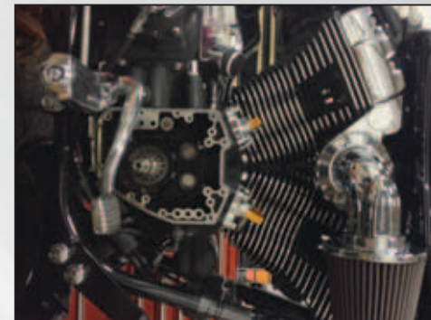
FIG 2 Camshaft plate, camshafts and oil pump removed.
