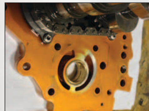
Fig 4 Cam plate damage and damaged crank bushing
