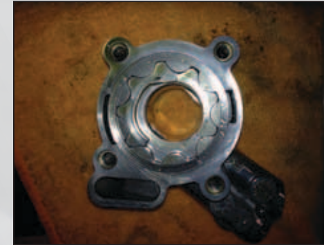
Fig 5 Destroyed oil pump ... Look closely and you will see the rotor is partially gone, and as of now the broken pieces are nowhere to be found ... not cool, not cool at all.
