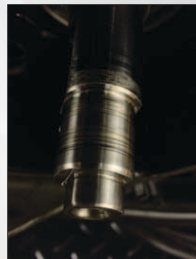
Fig 3 Crank End Damage
