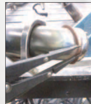
FIG 6 Removing old exhaust flange
