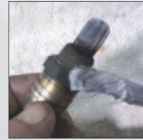
FIG 7 Coating the O2 sensor threads with anti-seize
