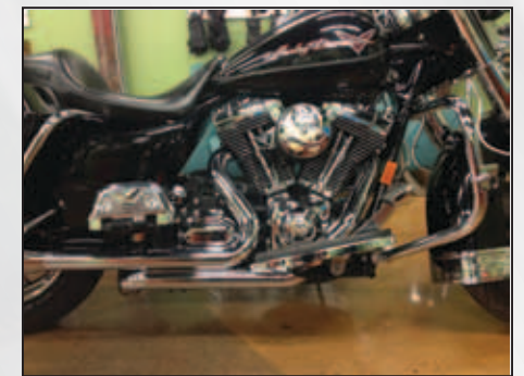
FIG 12 New exhaust right side
