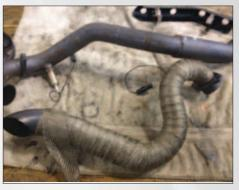
FIG. 2 Practice Wrap (dry wrap) you can see all the bends, sensors, tabs and how they affect the tape.
