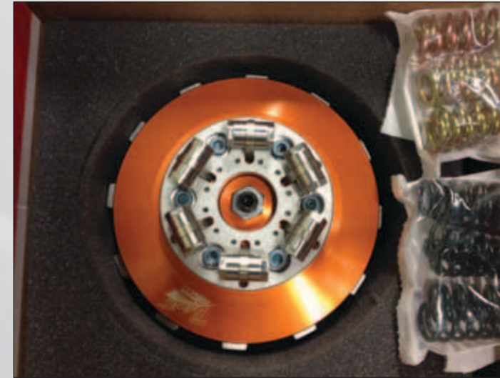
Fig 3 Barnett lock up clutch (fits under stock cover)
