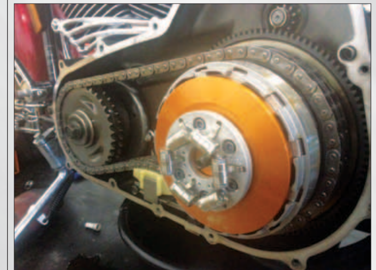
Fig 5 Lock-Up Clutch installed!! Wheelie Time!!!!
