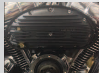
Fig 6 Plenum installed, the blow-off valve connection is on the lower left side of the plenums heat exchanger cover, there is a sneaky bolt behind that blow-off valve vacuum fitting.
