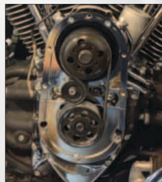
Fig 4 Lower unit, upper unit with blower, belt and tensioner installed (notice the 2 oil lines behind unit on right)
