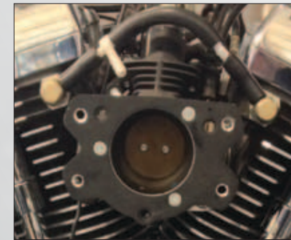
Fig 5 Adaptor plate and Vacuum lines installed
