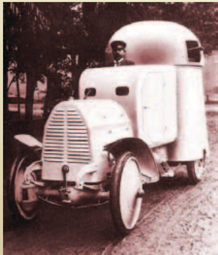
Austro-Daimler armored-car with four powered wheels. It was first demonstrated during maneuvers of the Austrian army in 1906. It was turned down because Emperor Franz-Josef said it was unsuitable for military use since "it would frighten the horses".
